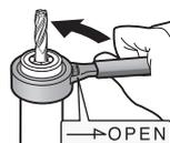
※ To ease the application of the MEGA WRENCH to the chuck it is suggested to rotate in the reverse direction while sliding into position.
