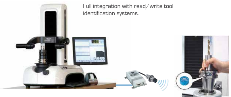
Integration via RS232 connection with your NC machine control.
