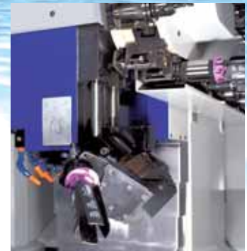
Clean-Tec may be utilized in all horizontal and vertical machining centers by using a normal chuck with clamping diameter 20 mm or 3/4".
