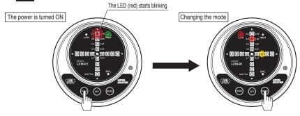
(a) Adjust the level in order to turn on the LED (blue) of the central position in the LOW mode. When the LED (blue) turns on, the inclination is within 0.1.
