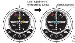
Adjust the level of the reference surface in order to obtain an inclination within 0.1 for both axes.
