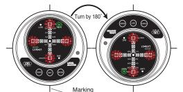
②Rotate the device by 180° using as reference the markings on the reference surface.
