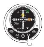
Adjust the level in order to turn on the LED (blue) of the central position.
